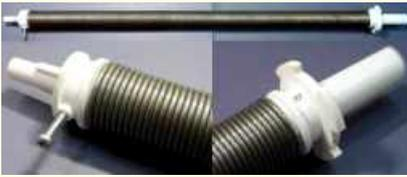
Spring assist for 38mm roller, left side /right side operation w/spring dim.1.8mm, length:430mm/630mm
